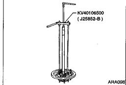
10. Remove wheel bearing together with bearing cage and baffle plate from axle shaft.
